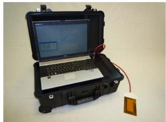
Systemcomponents: Evaluation Unit, Measurement device with current source, Hot Foil Sensor
