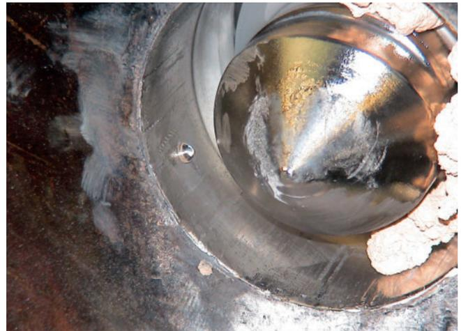
Fig. 2. The tip of the measuring probe extends into the extruder to ensure that the lens is covered with melt
